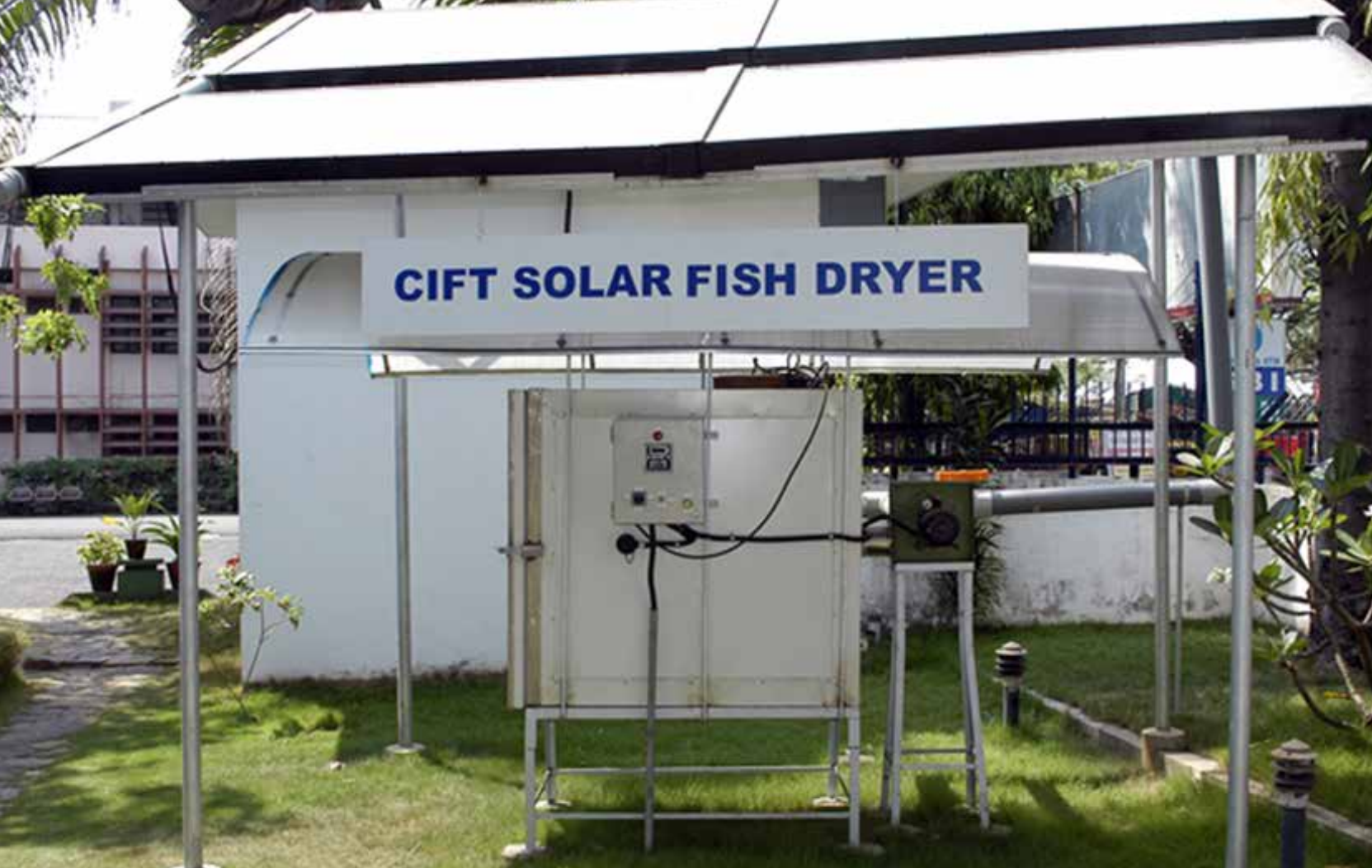
Fig1: CIFT solar hybrid fish dryer with electrical backup system
