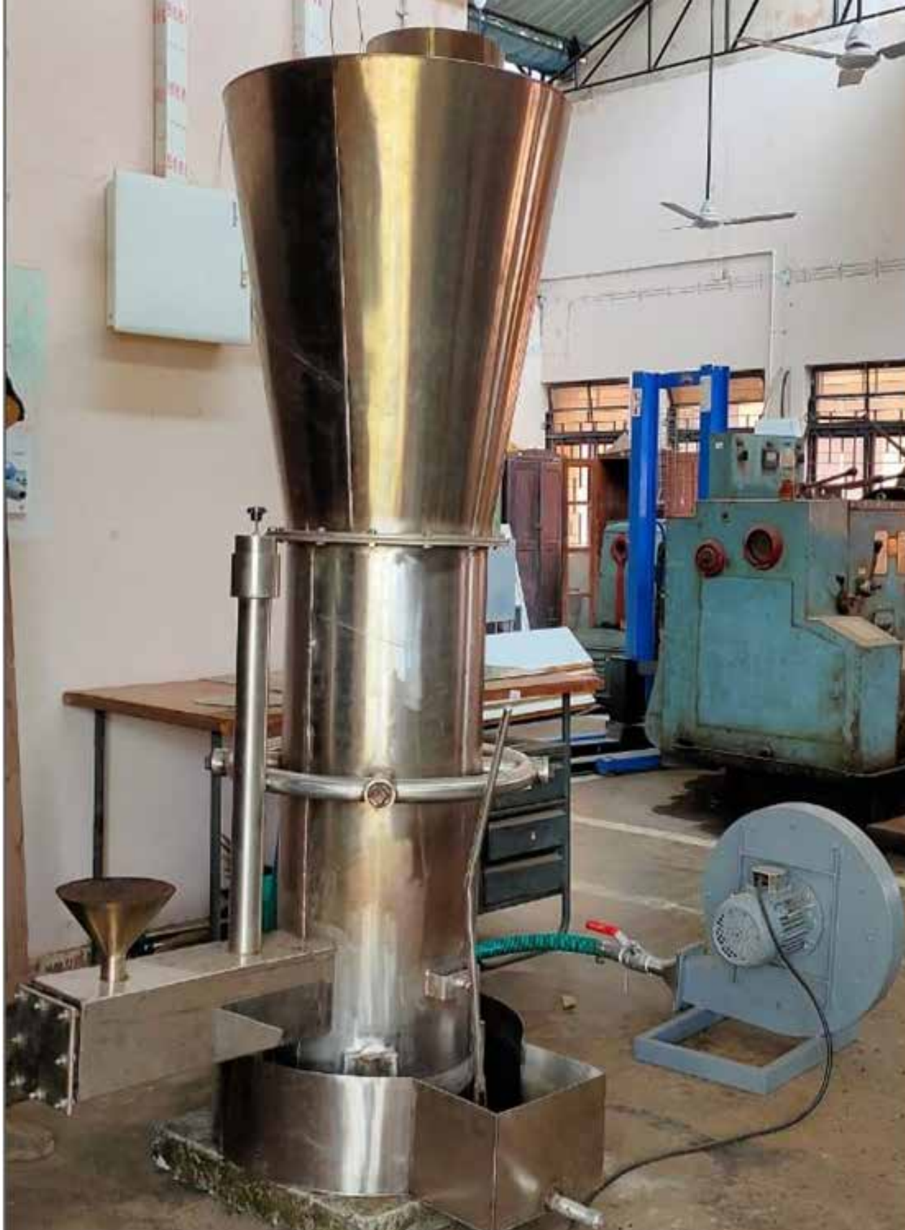
Fig 3: Biomass gasifier system with blower assembly
