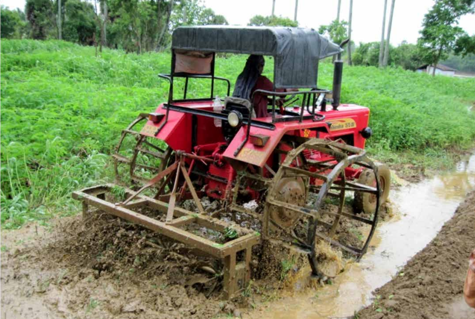
Fig. 2 KAU Helical blade puddler
