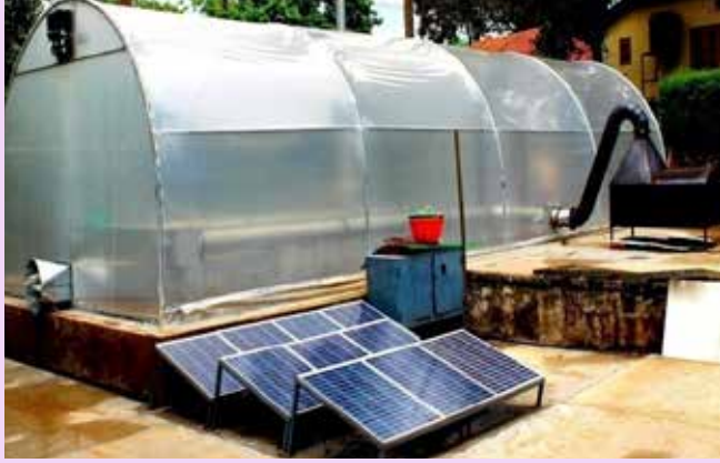
Fig. 2 a) Solar tunnel dryer installed at ICAR – IISR, Kozhikode b) Drying of mace in solar tunnel dryer
