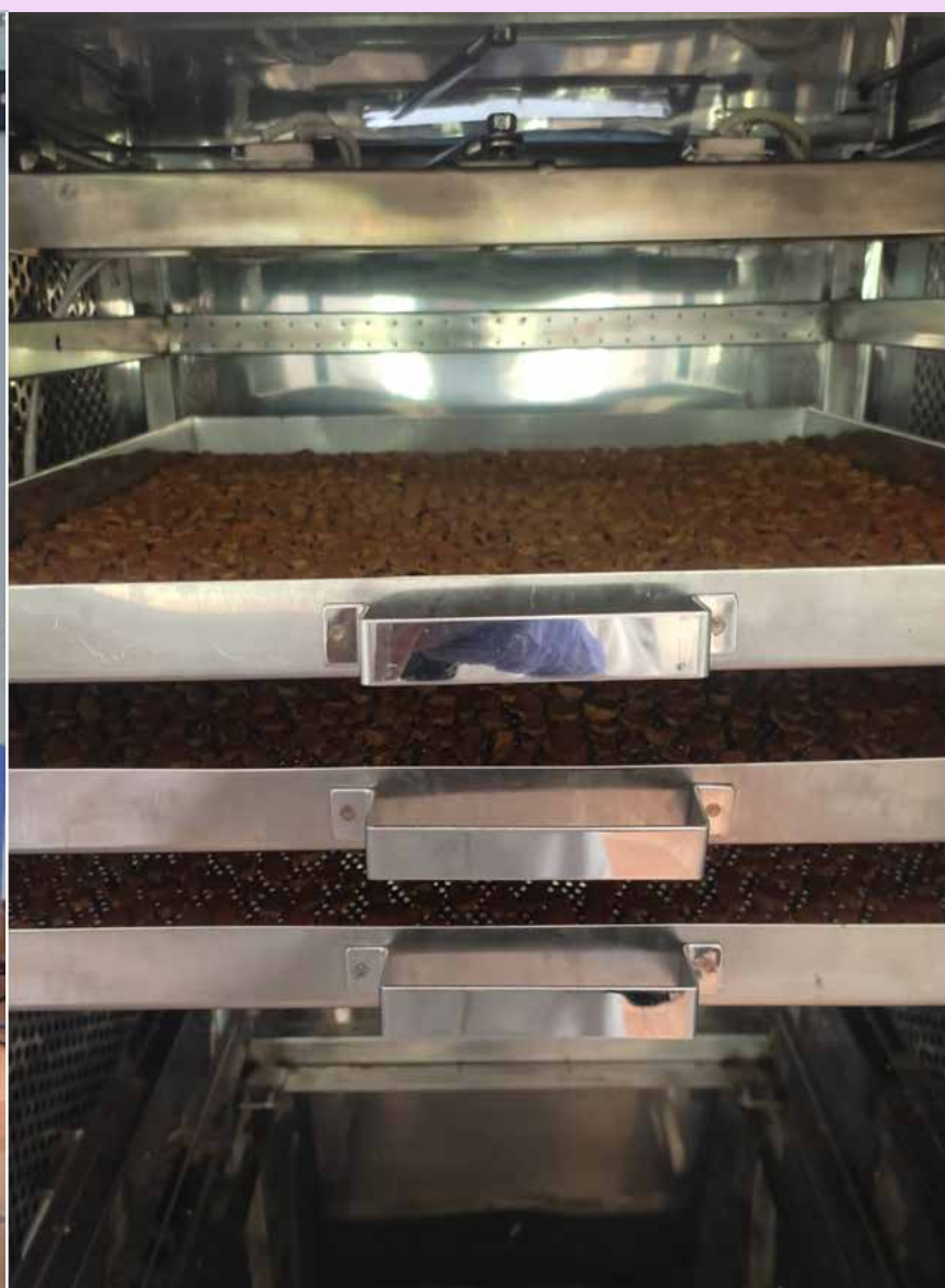
Fig. 9 a) Infrared dryer installed in ICAR – IISR, Kozhikode b) Drying of turmeric slices in infrared dryer
