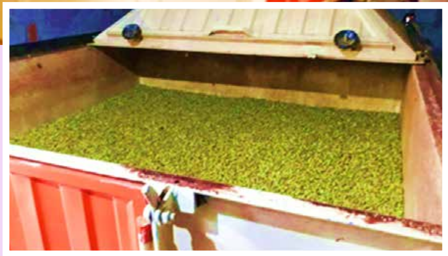
Fig. 3 Biomass drying of cardamom (Source: Greenguard dryers, Idukki)
