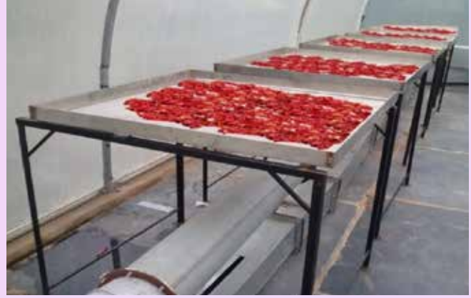
Fig. 2 a) Solar tunnel dryer installed at ICAR – IISR, Kozhikode b) Drying of mace in solar tunnel dryer
