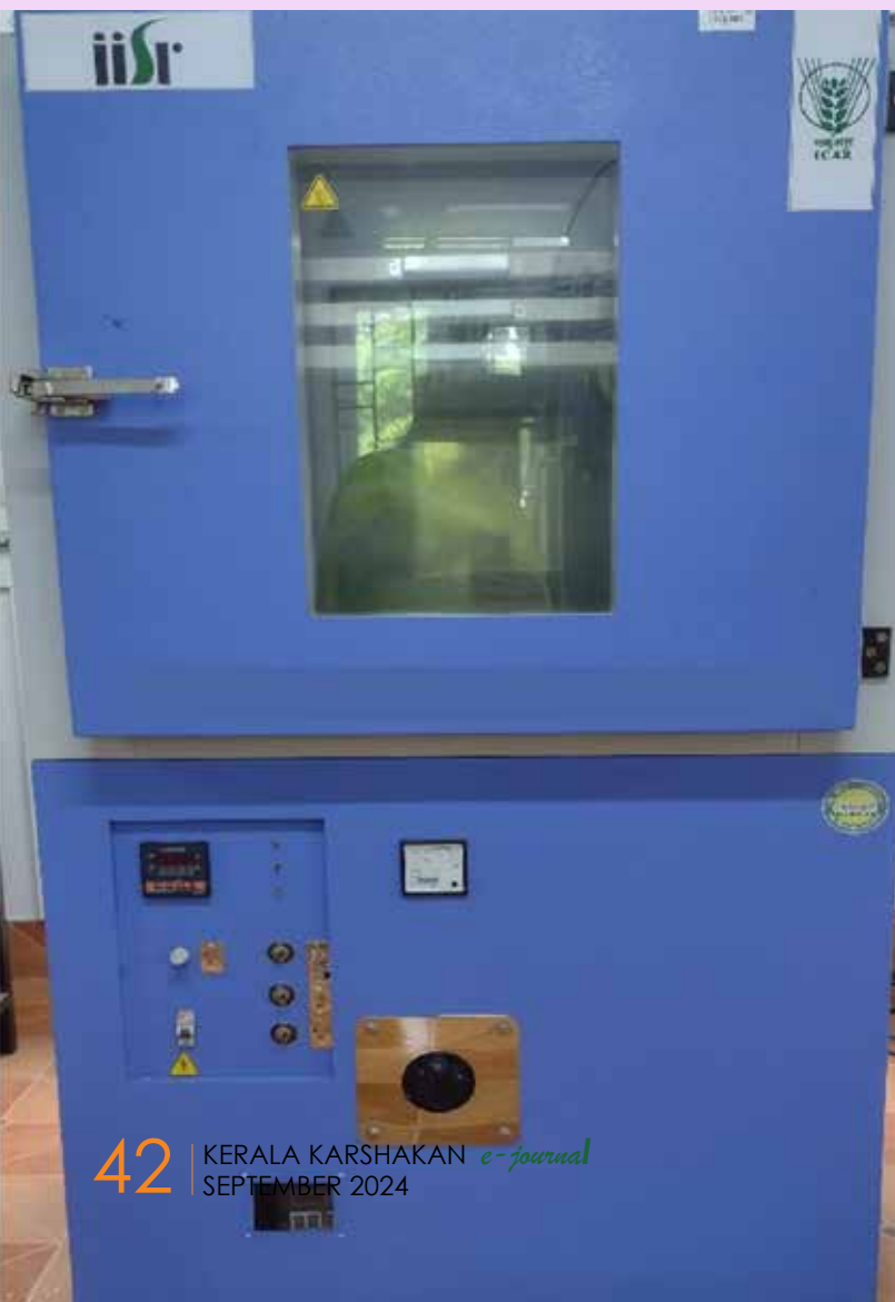
Fig. 9 a) Infrared dryer installed in ICAR – IISR, Kozhikode b) Drying of turmeric slices in infrared dryer
