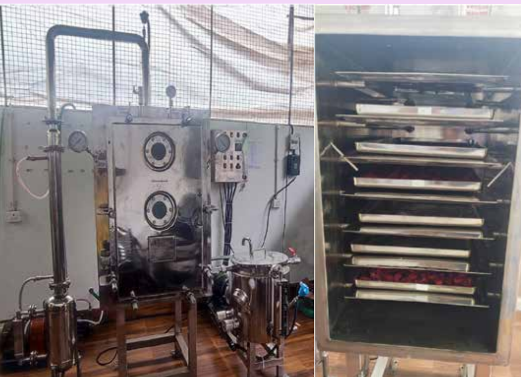
Fig. 7 a) Vacuum tray dryer installed at ICAR – IISR, Kozhikode b) Drying of mace in vacuum tray dryer
