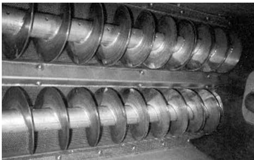
Steam heating chamber of F.V.E process.
